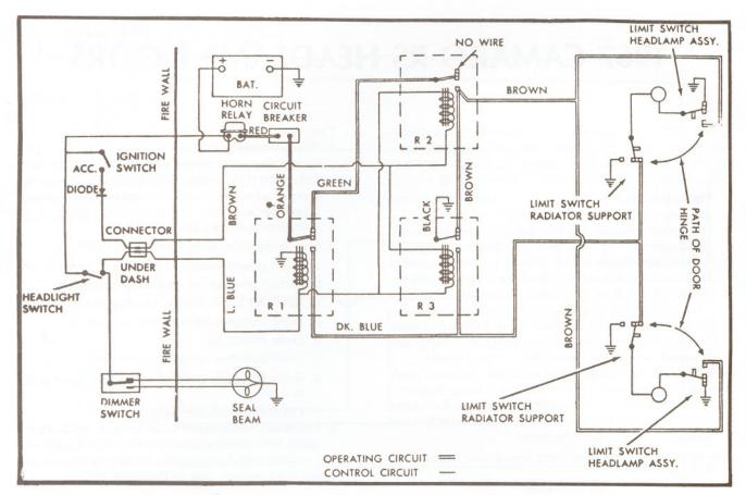
Camaro Headlamp Door Wiring-System in "Closed" Position
