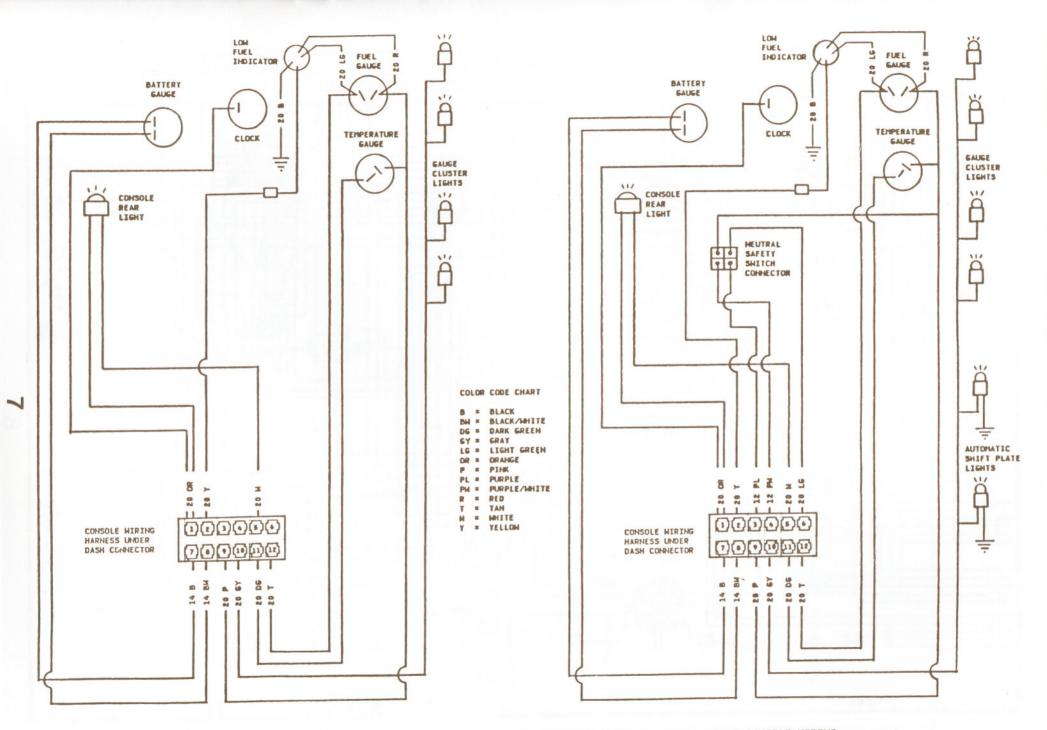
1967 CONSOLE WIRING AUTOMATIC TRANSHISSION WITH CONSOLE GAUGES
